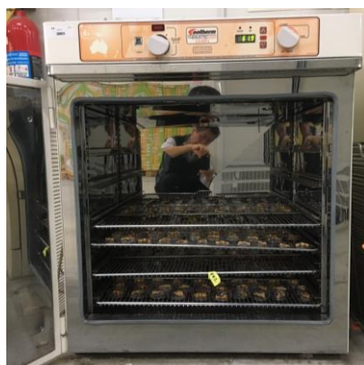
Figure 5. A drying oven like this offers even and more predictable drying.
